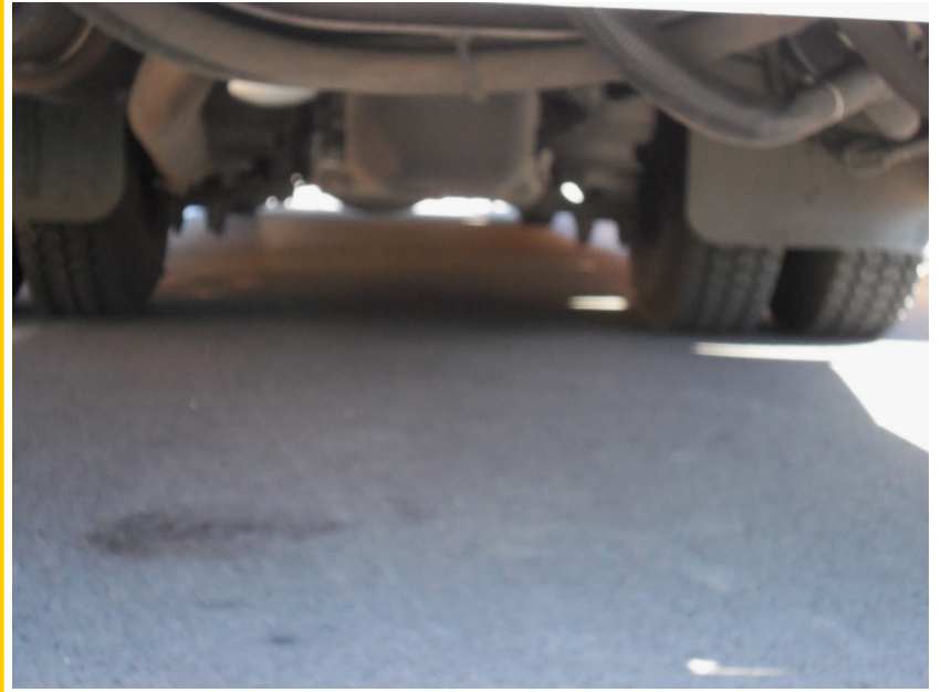
LEAKS UNDER BUS
