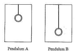
Pendulum A has a string, which is 4 inches long. Pendulum B's string is 8 inches long. The washer attached to both is 2 inches in diameter and weighs 3 grams. Students count how many times the pendulum will swing back and forth in 15 seconds.
