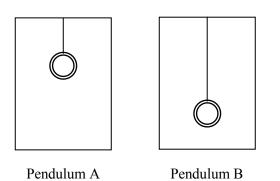
Pendulum A has a string, which is 4 inches long. Pendulum B's string is 8 inches long. The washer attached to both is 2 inches in diameter and weighs 3 grams. Students count how many times the pendulum will swing back and forth in 15 seconds.
